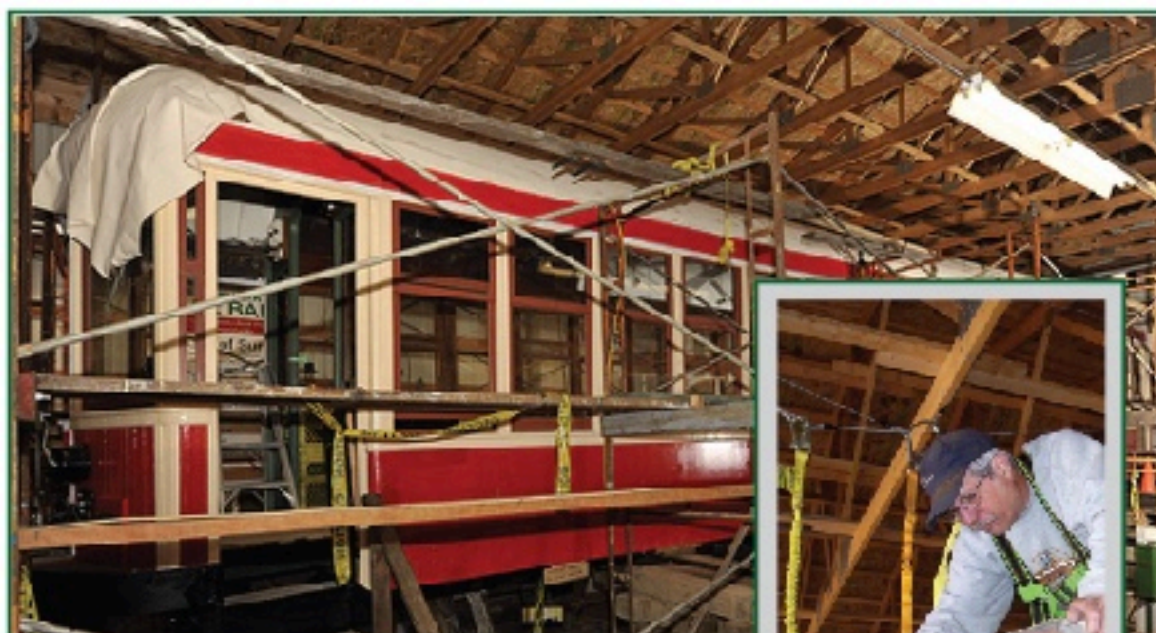
New roof membrane being applied by Robert Ashton
