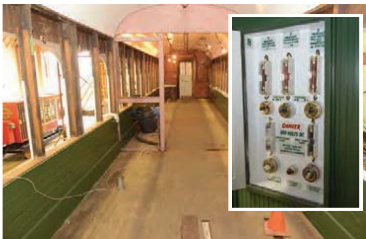
BCER 1304 interior; needs repainting along with the floor. The electrical panel (inset) have been rebuilt and refinished.
