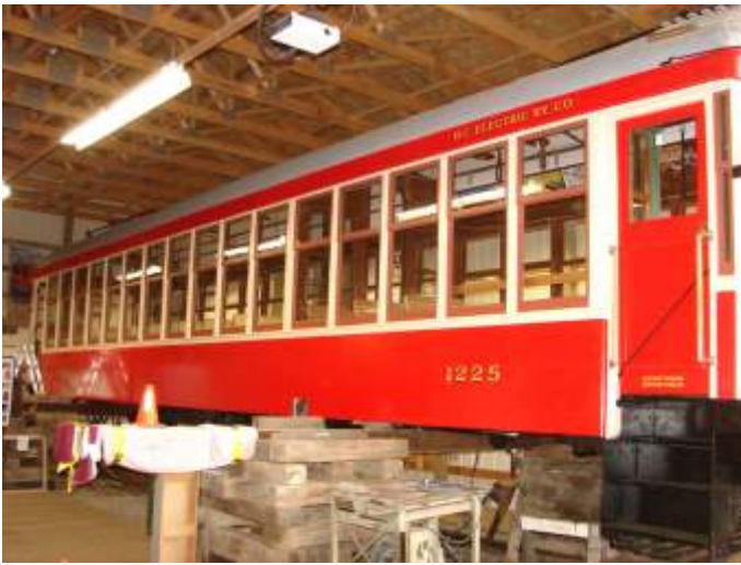
Side view of 1225 sitting on jacks awaiting the return of the trucks from Carr's Machining - see page 7
