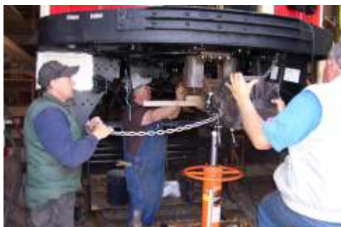
Reconditioning the wooden seats and re-upholstering with rattan, and installing the coupler at the "A" End
