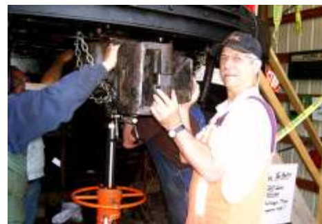
Reconditioning the wooden seats and re-upholstering with rattan, and installing the coupler at the "A" End
