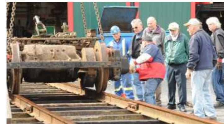
Delicate moves to place the trucks on the track
