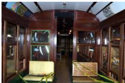
Inside, the ceiling panels and woodwork is coming into place, including the "B" End at right
