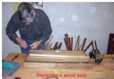
Reconditioning the wooden seats and re-upholstering with rattan, and installing the coupler at the "A" End
