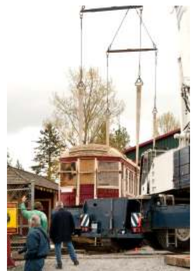
The sixty foot car body is hoisted over the fence (right)
